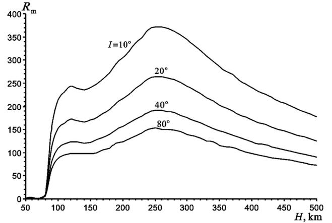
**Figure 5.** Dependence of the efficiency parameter  $R$  on the height  $H$  of the source for different latitudes in the daytime ionosphere ( $f = 0.5$  kHz).
