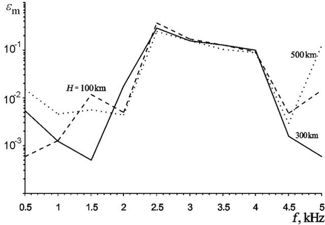
**Figure 3.** Frequency dependence of the relative error for daytime ionosphere ( $H = 100, 300,$  and  $500$  km).
