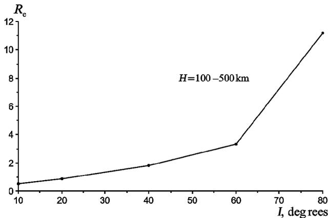
**Figure 8.** Dependence of the efficiency parameter  $R$  on latitude for the heights of the source  $H = 100 - 500$  km for the daytime and nighttime ionosphere ( $f = 0.5$  kHz).
