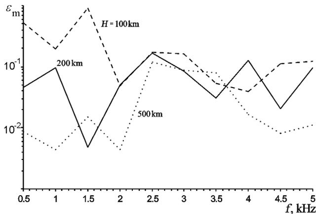
**Figure 4.** Frequency dependence of the relative error for nighttime ionosphere ( $H = 200, 300,$  and  $500$  km).
