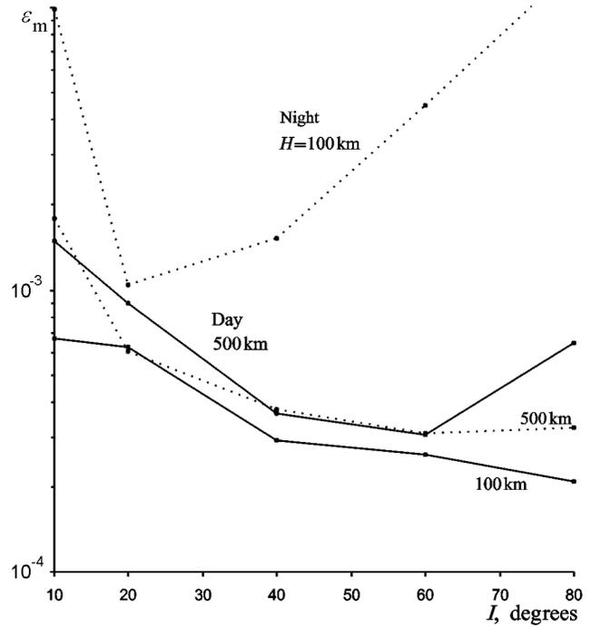
**Figure 9.** Dependence of the relative error on latitude for the heights  $H = 100$  and  $500$  km for daytime and nighttime ionosphere ( $f = 0.5$  kHz).
