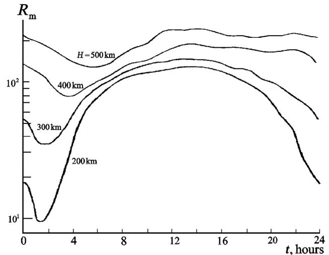
**Figure 10.** Daily variations of the efficiency parameter  $R$  for different heights  $H$  of the source ( $f = 0.5$  kHz).
