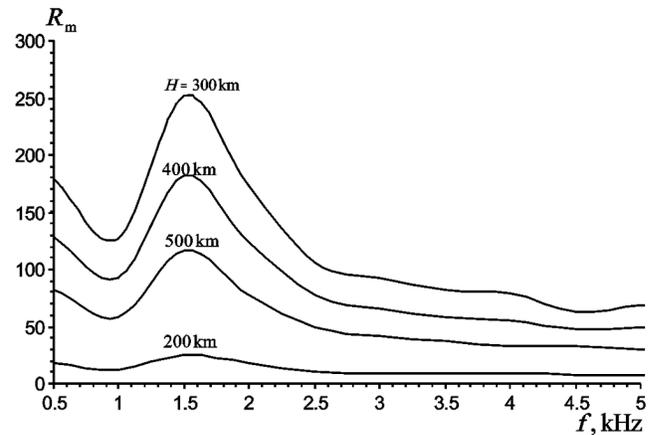
**Figure 2.** Frequency dependence of the efficiency parameter for different heights  $H$  of the source in the nighttime ionosphere.
