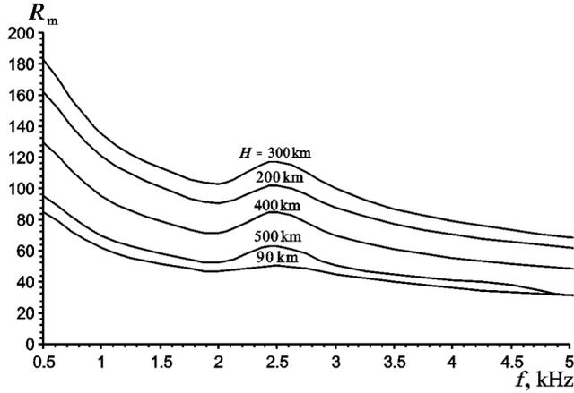
**Figure 1.** Frequency dependence of the efficiency parameter for different heights  $H$  of the source in the daytime ionosphere.
