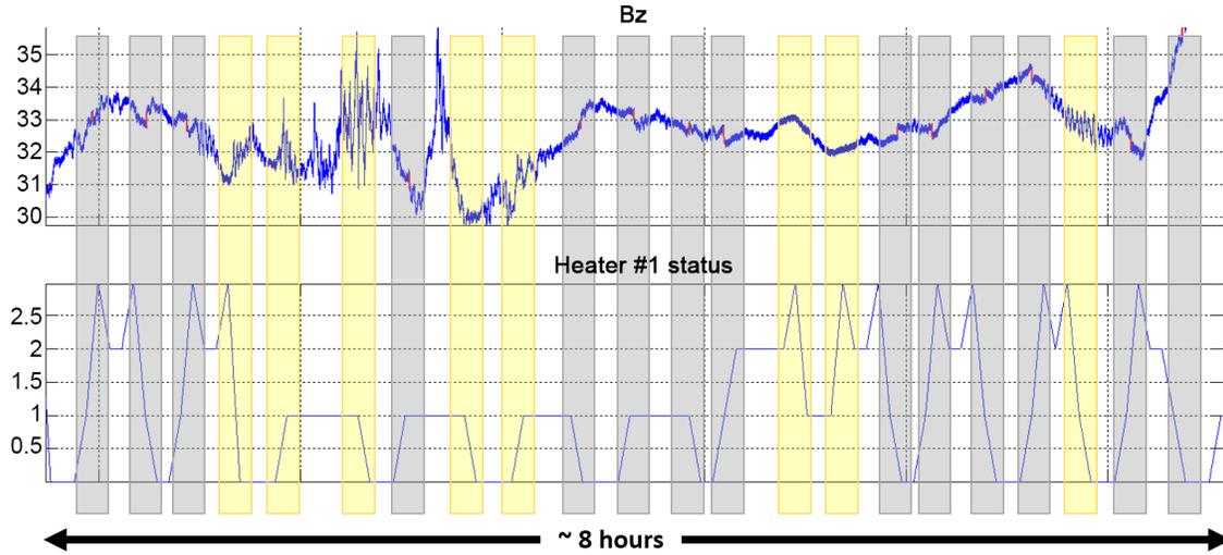
**Figure 7.** Examples of jump detection using JM algorithm. The original magnetogram is given on the upper plot; recognized jumps are marked with red. The lower plot provides the heater status information within the same period. Vertical rectangles outline the heater transition state between “on” and “off”. Grey rectangles correspond to correlation between jumps and heater switches. Yellow rectangles correspond to correlation absence, i.e. no jumps associated with heater switches.
