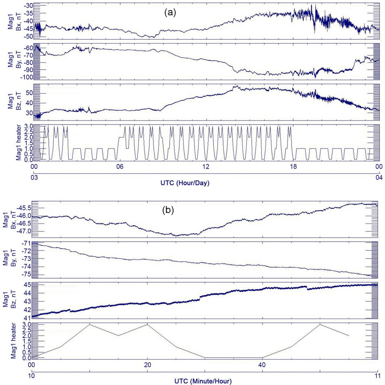
**Figure 6.** 1-day plot (3 April 2010) (a) and 1-hour plot (1000–1100 UTC, 3 April 2010) (b) plots of 2 Hz magnetograms ( $B_x$ ,  $B_y$ ,  $B_z$ ) and heater status. Heater status changes are step-wise as captured in 5-minute housekeeping packets.
