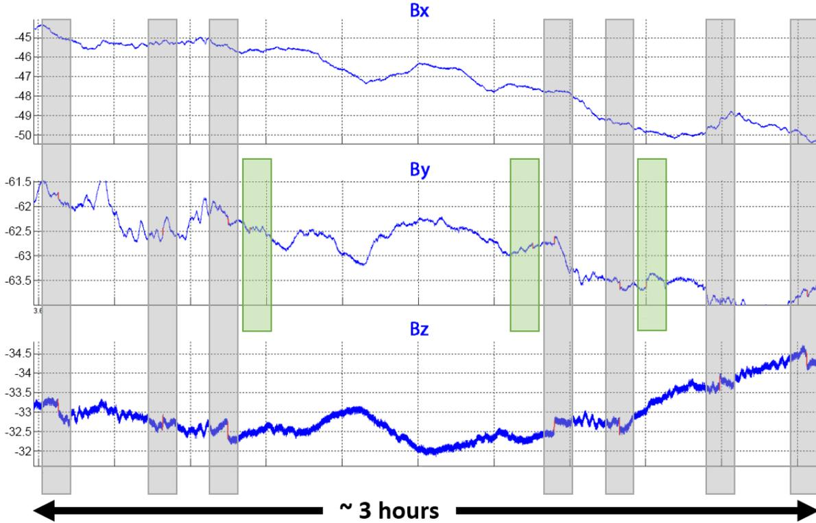
**Figure 9.** Jump recognition results for each component  $B_x$ , (upper plot),  $B_y$  (middle plot) and  $B_z$  (lower plot).  $B_x$  component does not contain jumps. Grey rectangles outline the simultaneous occurrence of jumps in  $B_y$  and  $B_z$  components; green rectangle outline jumps, which are present in the  $B_y$  component only.
