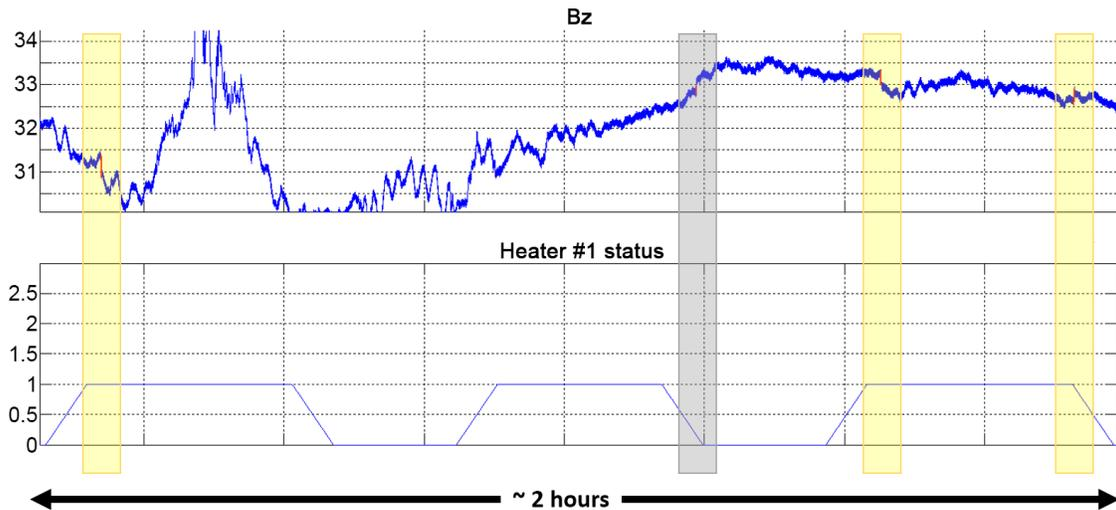
**Figure 8.** Examples of jump detection using JM algorithm. The legend is the same as in Figure 7. This example shows that jump occurrence is not necessarily associated with heater switches (yellow rectangles).
