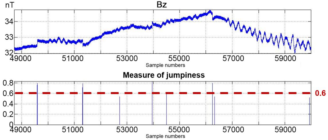
**Figure 1.** Original time series (upper panel) and derived measure of jumpiness (lower panel). The  $\beta$  parameter of the JM algorithm is taken as 0.6 indicated by the red dashed line.
