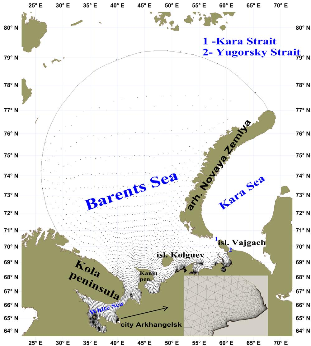
Figure 1. Calculated unstructured mesh for modeling.
