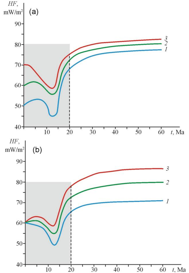
**Figure 6.** Surface heat flow evolution over the middle point of uplift. (a) Top picture shows the influence of different conductivities  $\lambda$  ( $L_a$ ): 1–2.0 (low), 2–2.5 (normal), 3–3.0 (high) W/m K. (b) Bottom picture shows the influence of different heat production rates  $H$ : 1–1.5 (low), 2–2.0 (normal), 3–2.5 (high)  $\mu\text{W}/\text{m}^3$ . Shaded area marks the time of shortening.
