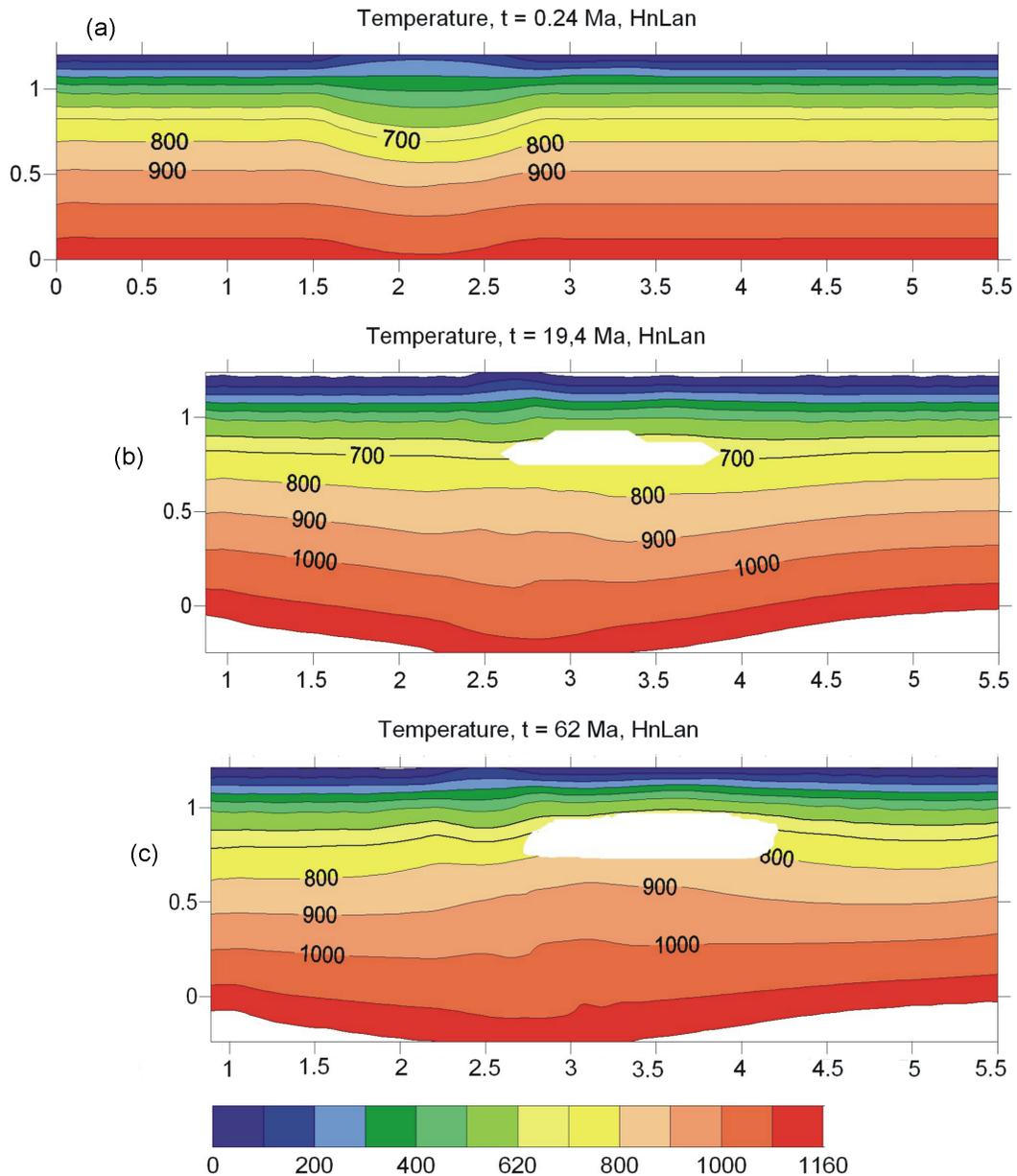
**Figure 4.** Temperature distribution for “normal” crust at: (a) – the beginning of deformation process, (b) – the end of collision process with a rate of 0.5 cm/yr and (c) – postcollision stage. Heat generation rate ( $H_n$ ) is  $2.0 \mu\text{W}/\text{m}^3$ , thermal conductivity  $\lambda (La_n) = 2.5 \text{ W}/\text{m K}$  for the upper crust. Horizontal and vertical scales 1 = 100 km. Blanked areas show approximate position of partial melting zone for “wet granite solidus” [Perchuk, 1973].
