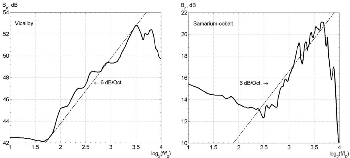
Figure 5. The distribution of noise at the outputs of the quartz magnetometers.
