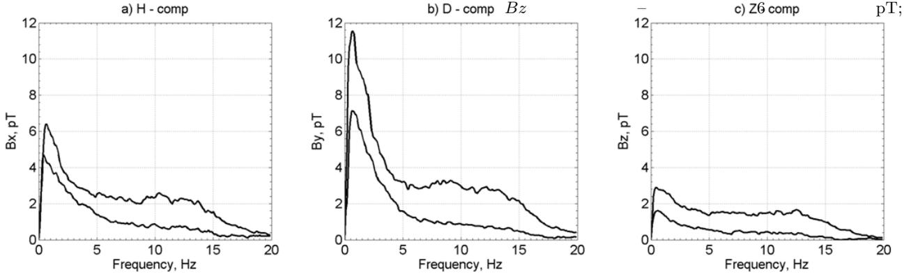
Figure 3. The noise spectra on outputs of quartz sensors.
