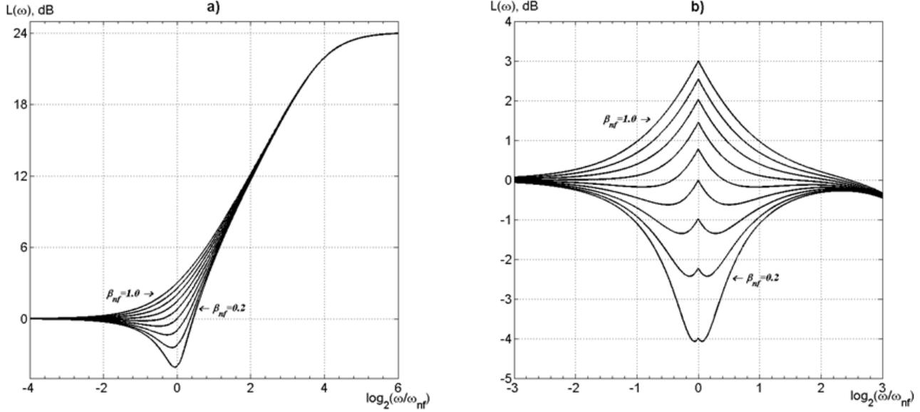
**Figure 1.** a) L AFC of a sensitivity threshold of the magnetometer; b) real L AFC of noise of a variometer at  $0.4 < \beta_{\text{nat}} < 0.7$ .
