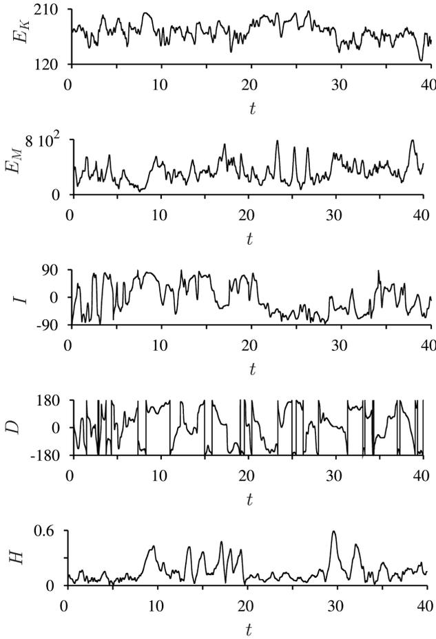
**Figure 1.** Evolution of the mean over volume kinetic  $E_K$  and magnetic  $E_M$  energies, inclination  $I$ , declination  $D$  and dipole intensity  $H$  at  $r_o$  for  $Ra = 550$ ,  $Pr = 1$ ,  $E = 0.03$ ,  $q = 20$ .
