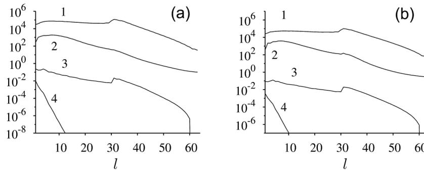
**Figure 5.** Spectra of the magnetic (1) and kinetic (2) energies in the liquid core, the Mauersberger-Lowes spectrum at the liquid core surface (3) and at the surface of the Earth (4) for  $Ra = 400$  (a) and  $Ra = 600$  (b).
