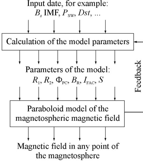
**Figure 1.** Schematic diagram of the Paraboloid model.  $R_1$  is the distance to the subsolar point,  $R_2$  is the distance to the earthward edge of the tail current sheet,  $\Phi_{PC}$  is the magnetic flux in the polar cap,  $B_R$  is the ring current intensity,  $I_{FAC}$  is the intensity of the Region 1 field-aligned currents,  $S$  is the flaring of the paraboloid of revolution (magnetopause).
